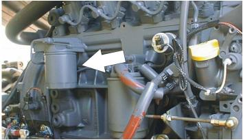
Lube Point(s) - Fill Cap/Spin-on Element (JLG P/N 7016331) Capacity - 6.3 qt (5.9 L) engine only Lube - EO Interval - Every Year or 1200 hours of operation
