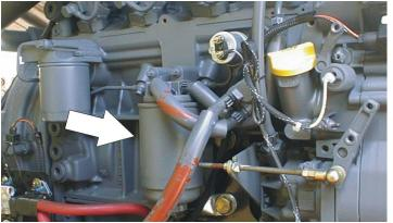
Lube Point(s) - Replaceable Element Interval - Every Year or 600 hours of operation
