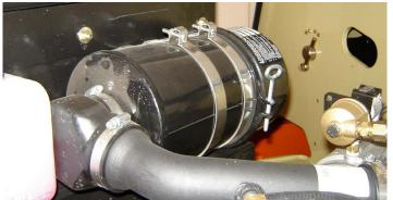
Lube Point(s) - Replaceable Element Interval - Every 6 months or 300 hours of operation or as indicated by the condition indicator 28. Air Filter - Deutz D2.9
