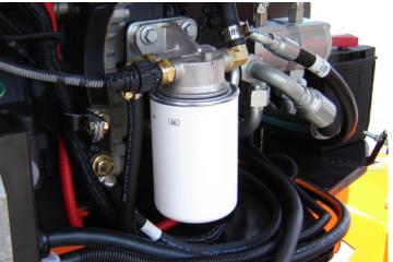
Lube Point(s) - Replaceable Element Interval - Drain water daily; Every year or 600 hours of operation
