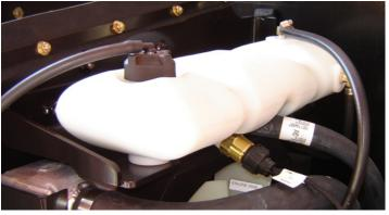
Lube Point(s) - Fill Cap Capacity - 3.2Gallon (12.1 L) Lube - Anti-Freeze Interval - Check level daily; change every 1000 hours or 2 years, whichever comes first
