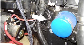
Lube Point(s) - Fill Cap/Spin-on Element (JLG P/N 7027965) Capacity - 4.5 qt (4.25 L) w/filter Lube - EO Interval - 3 Months or 150 hours of operation Comments - Check level daily/Change in accordance with engine manual 13. Oil Change w/Filter - Isuzu
